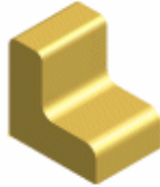
Figure 4 Filletting edges of angle part
