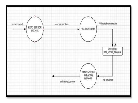
Fig. 2. Level 1 DFD (Data Flow Diagram)
