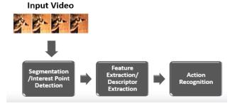
Fig. 2. General steps involved in representation-based methods
