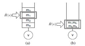
Fig. 2. Messages in the queue of node v with and without aggregation. Without aggregation, when node v is scheduled, the message m1 will be forwarded. With aggregation, all messages are aggregated into a single packet and will be forwarded simultaneously. (a) Without in- network aggregation. (b) With in-network aggregation.
