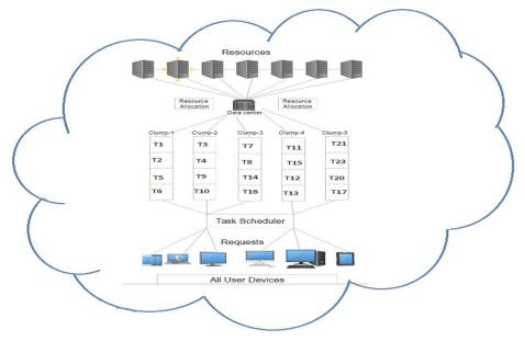
Fig. 2. Architecture of task-clumping schedule model
