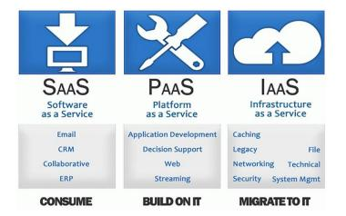
Fig. 1. Separate Services of Cloud Computing
