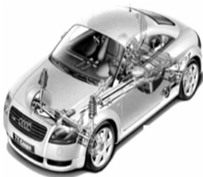
Fig. 6 .Audi TT Coupe with hydroformed rear axle components [22]
