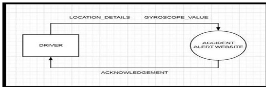
Fig. 1. Level 0 DFD (Data Flow Diagram)
