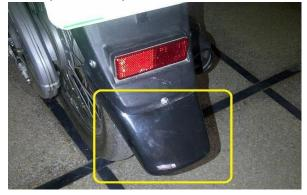
Fig.4.3 Mudguard with supplementary mudguard
