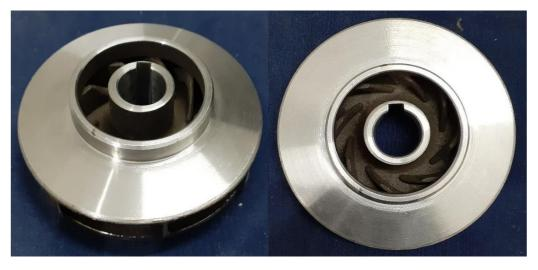
Fig. 3.0.1. Impeller manufacturing via sand casting method
